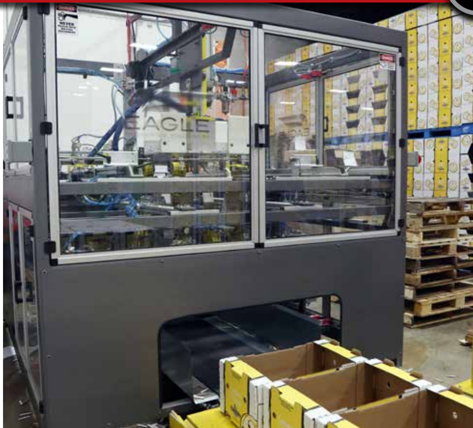
M.L. Catania uses a VassoyoAir automatic trayforming machine designed and manufactured by Eagle Packaging Machinery to pack lemons, limes and clementine fruits, as well as larger types of fruits such as grapefruit into the stackable corrugated trays.
