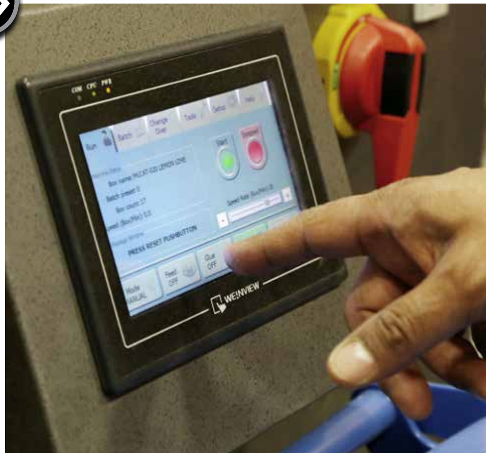
The HMI (human-machine interface) on the VassoyoAir trayformer manufactured by Eagle Packaging Machinery is easy to use, helping M.L. Catania employees easily alter glue patterns on corrugated tray blanks as required.
