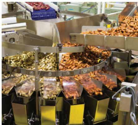
WeighPack's 24 head PrimoCombi multi-head weigher with three product mixing weighs product before it is bagged.
