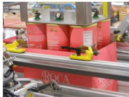
Eagle Packaging Machinery's Pick & Place Automation precisely loads each Roca container into the case while simultaneously orienting all logos to ensure that shipments are retail-ready.
