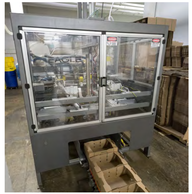
Supplied by WeighPack Systems and manufactured by Eagle Packaging Machinery, the high-speed VASSOYO Air trayforming system can achieve speeds of up to 25 cycles per minute at the Bercy Foods plant in Montreal.
