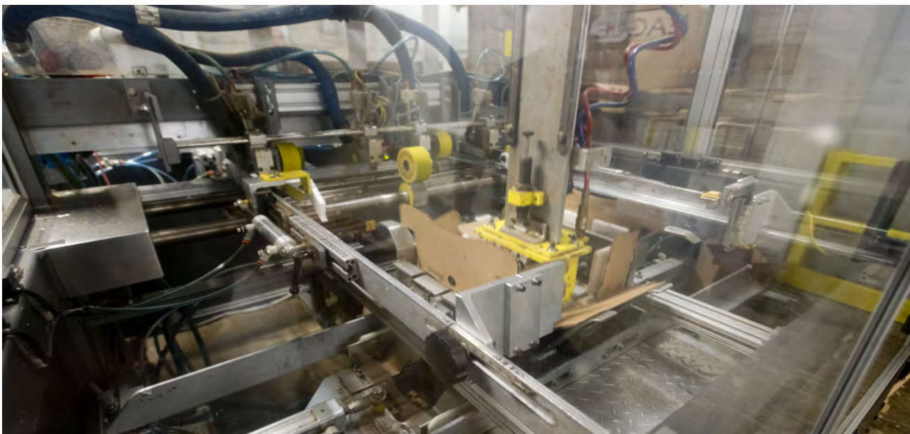
Supplied by WeighPack Systems and manufactured by Eagle Packaging Machinery, the high-speed VASSOYO Air trayforming system can achieve speeds of up to 25 cycles per minute at the Bercy Foods plant in Montreal.
