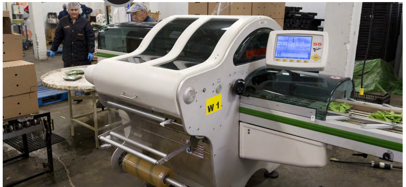
The Fabbri Model 55 Plus shrinkwrapping machine from Reiser can overwrap up to 55 containers per minute.
