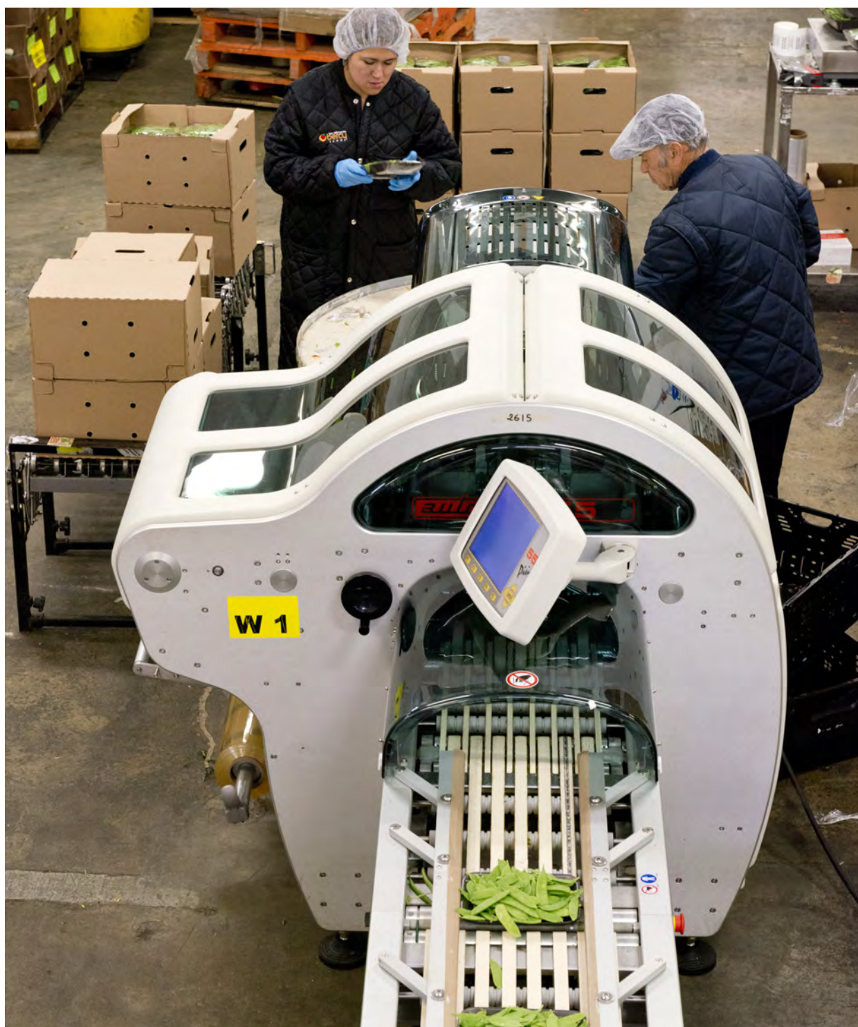
Bercy Foods uses a Fabbri Model 55 Plus shrinkwrapping machine from Reiser Canada to apply a clear film cover over its tray-packed fresh fruit and vegetable products at its state-of-the-art production facility in north-end Montreal.
